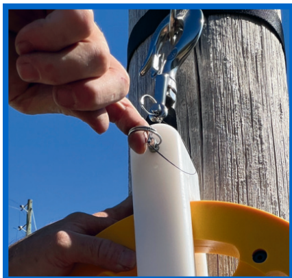
Remove retainer pin
