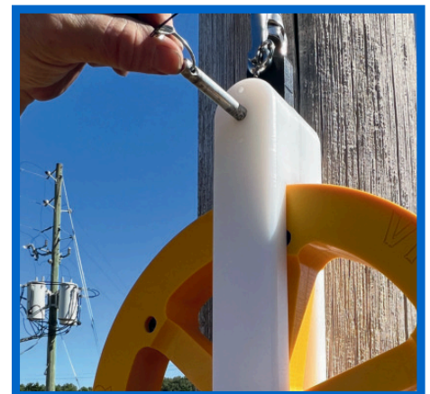
Re-insert retainer pin
