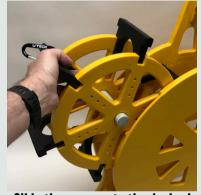
Slide the spacers to the desired spool diameter by removing the thumb screw and reinserting in the desired position.
