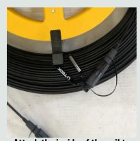
Attach the inside of the coil to the spool by using the carabiner (included) or tie wraps (not included).
